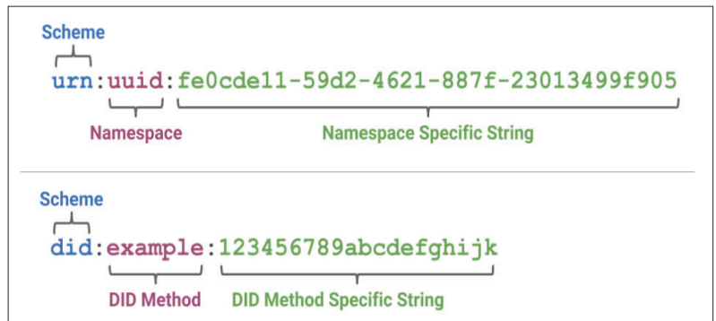
FIGURE 2. The structure of DIDs follows the same basic pattern as URNs.
